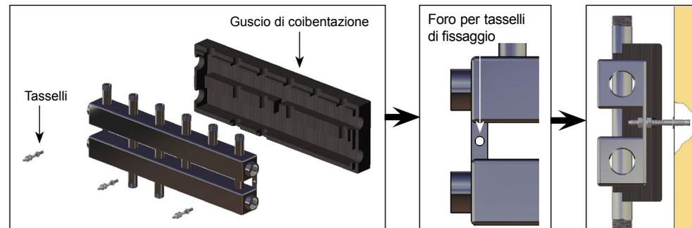
**INTERASSI DEI FORI PER IL FISSAGGIO**
